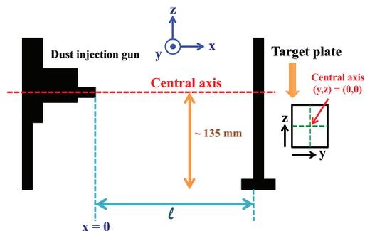
FIG. 2. Schematic view of the experimental setup.
