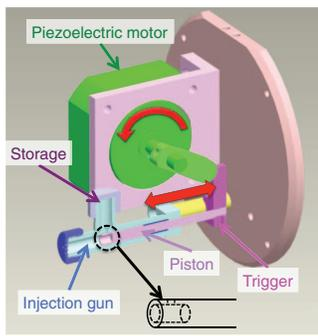
FIG. 1. Schematic view of the particle injection system.
