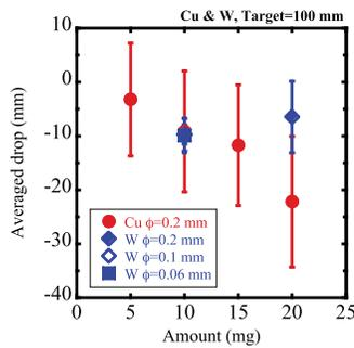
FIG. 4. Average drops as a function of the amount of Cu and W particles.
