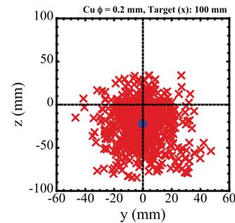
FIG. 3. Example of distribution of ejected Cu particles on the target plate and the average drop.
