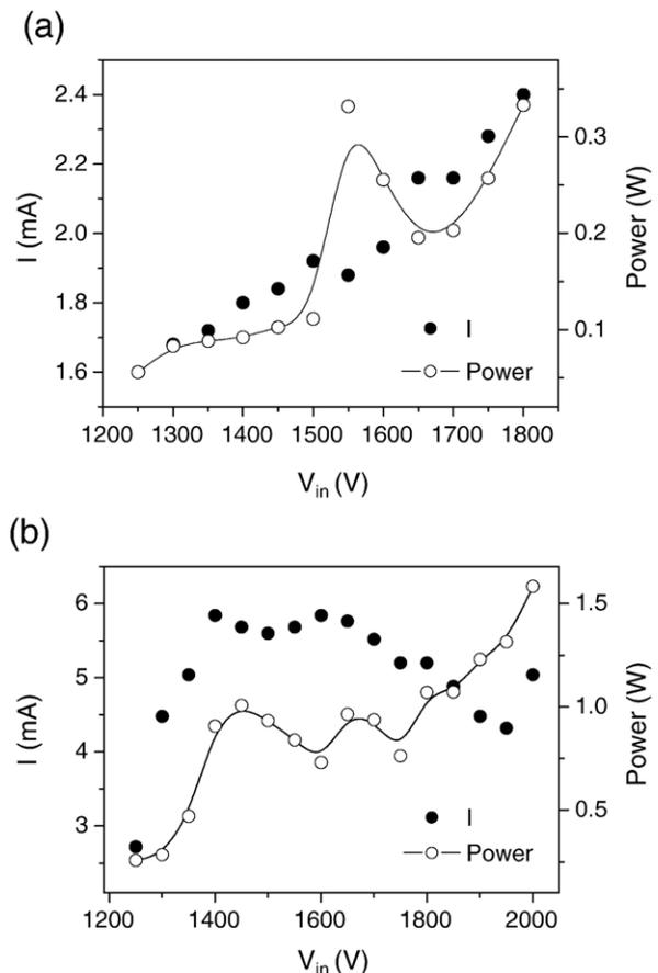
Fig. 2.  $I$ - $V$  characteristic curve and power dissipated to the plasma for a discharge source consisting of (a) pin to conducting plane electrode and (b) pin to conducting plane electrode with a dielectric barrier.
