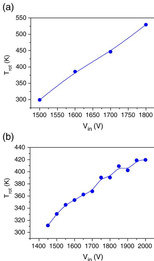
Fig. 3. Rotational temperature against the input voltage for a discharge source consisting of (a) pin to conducting plane electrode and (b) pin to conducting plane electrode with a dielectric barrier.
