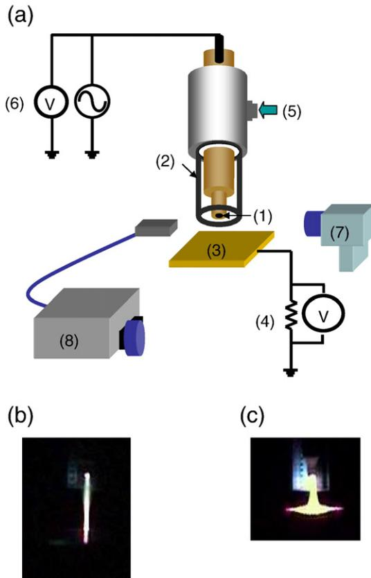
Fig. 1. (a) Experimental setup. Plasma images for a discharge source, consisting of (b) pin to conducting plane electrode and (c) pin to conducting plane electrode with a dielectric barrier.
