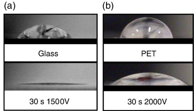
Fig. 4. Images showing the contact angle change for (a) glass and (b) PET before (upper) and after (lower) the plasma treatments for 30 s.
