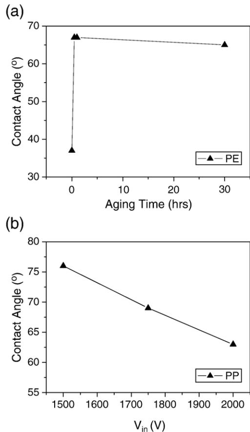
Fig. 6. (a) Change of the contact angle against the aging time for a polyethylene film. (b) Input voltage effects on the aging time for a polypropylene film 1 week after the plasma treatment.
