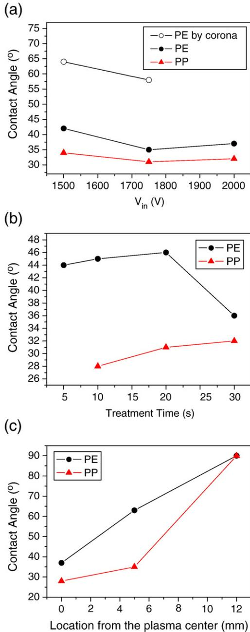
Fig. 5. Contact angle versus (a) input voltage, (b) treatment duration, and (c) treated location from the plasma radial center for polyethylene and polypropylene films.
