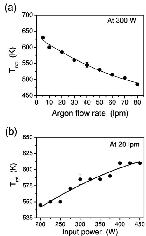
FIG. 5. Rotational temperature measured as a function of (a) argon flow rate (at 300 W), and (b) input rf power (at 20 lpm).  $T_{rot}$  decreases as flow rate increases due to more significant cooling by the introduced cold gas particles.  $T_{rot}$  increase as input power increases is attributed to more energy transfer from heated electrons to heavy neutrals.
