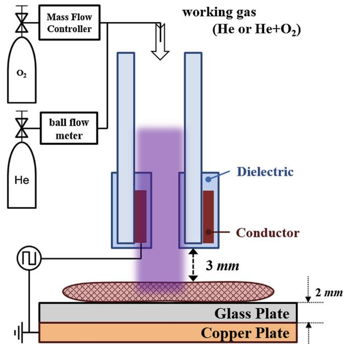
Fig. 1. Schematic diagram of the experimental setup for preparation of dielectric barrier discharge plasma.
