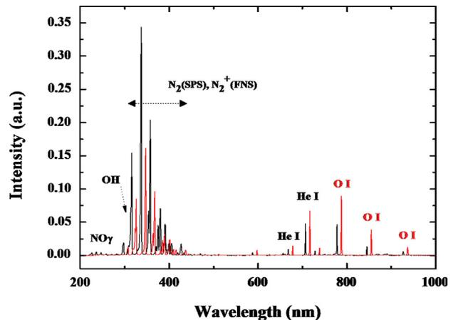
Fig. 2. A typical emission spectrum of the plasma. Helium atomic lines due to helium feeding gas, NO, OH,  $\text{N}_2$ ,  $\text{N}_2^+$  molecular spectra, and excited oxygen atomic emission lines due to the ambient air are observed. \*Black line: He, red line: He +  $\text{O}_2$ . (For interpretation of the references to color in this figure legend, the reader is referred to the web version of this article.)
