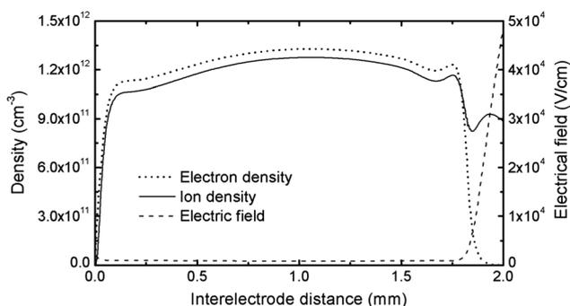
FIG. 2. Spatial profiles of electron density, molecular helium ion density and electric field across the interelectrode discharge gap at the time instant of discharge current peak with the bare electrodes.
