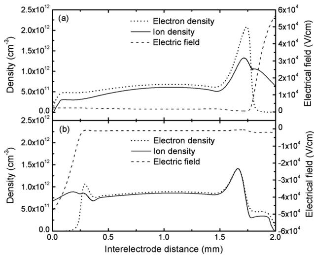
FIG. 5. Spatial profiles of electron density, molecular helium ion density and electric field across the discharge gap at the time instant of (a) the first discharge and (b) the second discharge current peak with the dielectric barrier electrodes.
