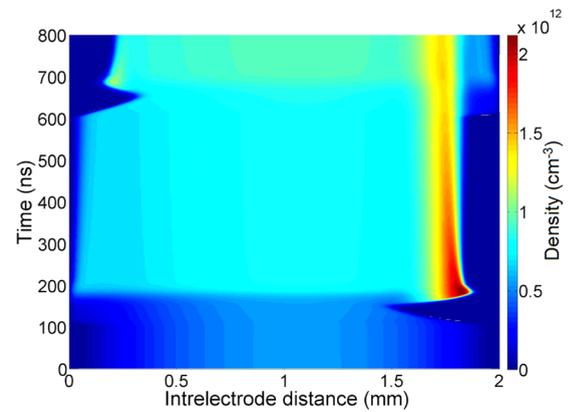
FIG. 6. Spatio-temporal evolution of electron density during the voltage pulse with the dielectric barrier electrodes.
