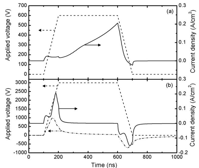
FIG. 1. Waveforms of applied voltage, gas voltage and discharge current density with (a) the bare electrodes and (b) the dielectric barrier electrodes.
