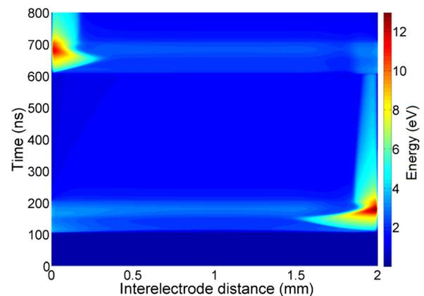
FIG. 7. Spatio-temporal evolution of mean electron energy during the voltage pulse with the dielectric barrier electrodes.
