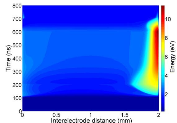
FIG. 4. Spatio-temporal evolution of mean electron energy during the voltage pulse with the bare electrodes.
