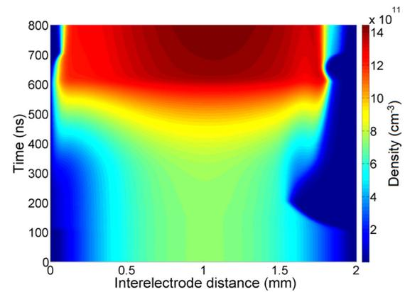
FIG. 3. Spatio-temporal evolution of electron density during the voltage pulse with the bare electrodes.
