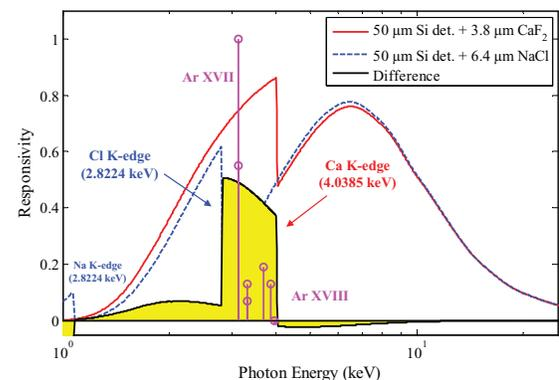
FIG. 4. Responsivity of the 50  $\mu\text{m}$  Si detector with a pair of Ross filters. The difference between the two spectra can be used as a bandpass filter.
