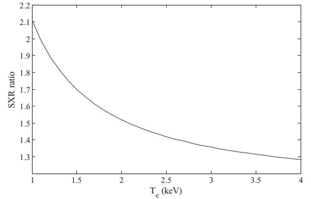
FIG. 3. Soft x-ray signal ratio as a function of  $T_e$ . Be filters of 10  $\mu\text{m}$  and 50  $\mu\text{m}$  are assumed.
