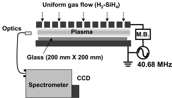
FIG. 1. Schematic illustration of the PECVD setup and optical instruments for plasma analysis.
