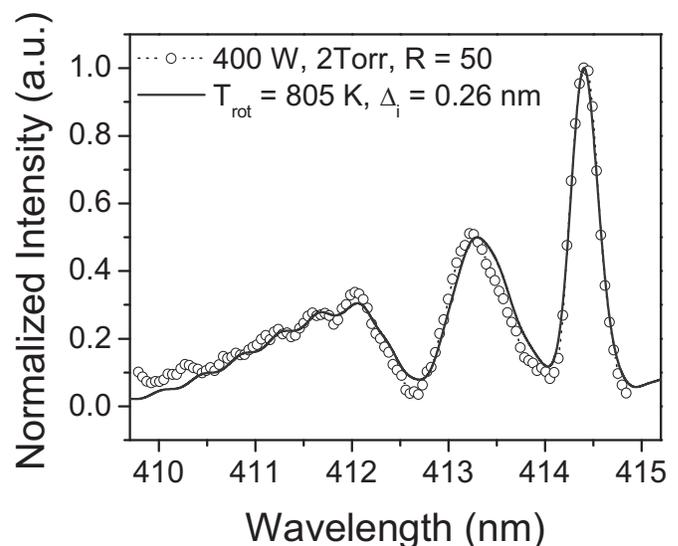
FIG. 3.  $T_{\text{rot}}$  obtained by the comparison between the experimental result ( $-o-$ ) and the synthetic spectrum ( $-$ ) of SiH (0,0) band is  $805 \text{ K}$ .
