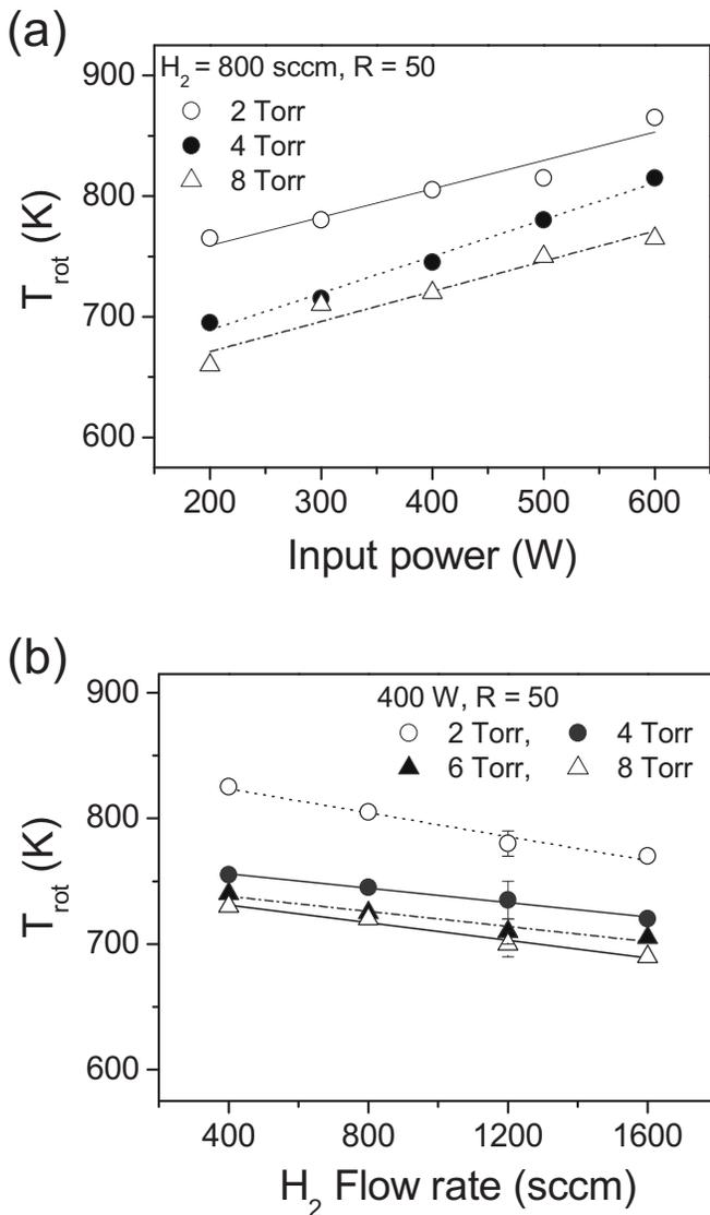
FIG. 4. (a) As the input power is increased,  $T_{rot}$  is also increased from 765 to 865 K at 2 Torr and 400 W, but (b)  $T_{rot}$  shows lower value at higher total gas flow rates because of gas cooling effects. In all cases of pressures, 2–8 Torr, the similar effects of input power and total gas flow rates are observed.
