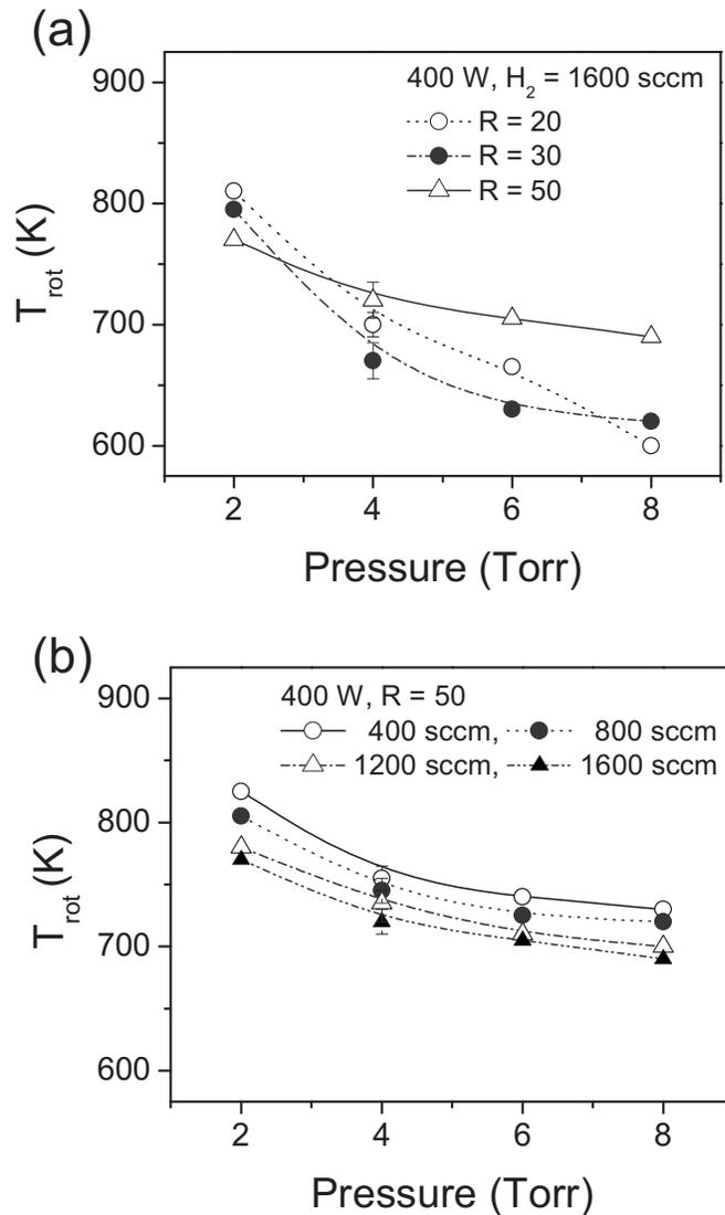
FIG. 5. (a) Gas pressure effects on  $T_{rot}$  for various  $H_2/SiH_4$  gas ratios (denoted as  $R$ ) and (b) for various total gas flow rate at 400 W. Increasing gas pressure,  $T_{rot}$  was decreased by frequent collisions between electron and neutrals.
