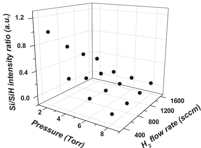
FIG. 6. Emission intensity ratio Si/SiH, which gives the information about electron temperature (Ref. 10), decreased as increasing gas pressure and total gas flow rate.
