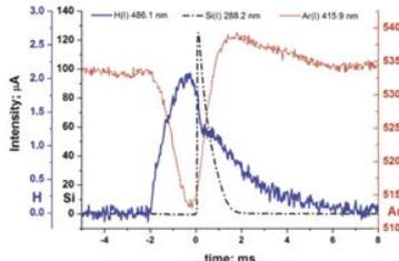
The intensities of the Si 288 nm, H 486 and Ar 416 lines measured simultaneously after the injection of 52 µm droplets of a 100 µg mL<sup>-1</sup> Si solution.
