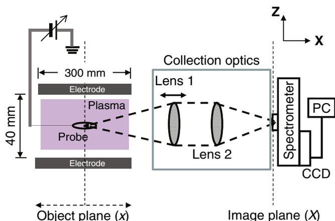
**Fig. 1.** Schematic of the experimental setup (side view, not in scale). The capacitive plasma was produced between the rectangular top and bottom electrodes (300 mm × 200 mm) with the gap distance of 40 mm. The plasma emission was measured in the X direction by moving Lens 1, while Lens 2 was used to focus the emission to the entrance slit of the spectrometer. A Langmuir probe was inserted inside the plasma to obtain electron temperature profile, i.e.,  $T_e(x)$ .
