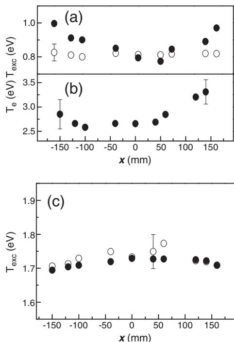
**Fig. 3.** (a) The spatial profile of (a) the excitation temperature without (open symbol) and with (closed symbol) the reconstruction, and (b) the electron temperature by a Langmuir probe. The operating condition was Ar 300 mTorr and 300 W at 90 MHz. (c) The excitation temperature profile without (open symbol) and with (closed symbol) the reconstruction at Ar 300 mTorr and 300 W at 13.56 MHz.
