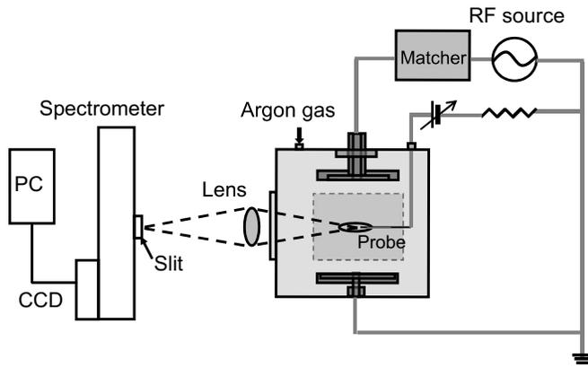
FIG. 1. Schematic of the experimental setup consisting of an OES system (spectrometer and a plano-convex lens) and a Langmuir probe. A lens of 500 mm focal length was used to focus the same diagnostic area of the probe measurement. The sampling area traced back to the plasma is a rectangle of  $0.05 \times 20 \text{ mm}^2$  of which location corresponds to that of the Langmuir probe.
