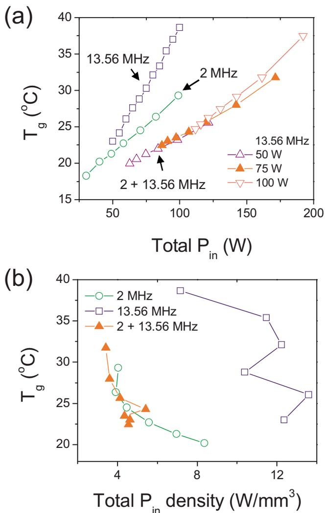
FIG. 4. (Color online) (a)  $T_g$  vs total input power and (b) total volume input power density. For the dual frequency case, 13.56 MHz  $P_{in}$  was fixed at (- $\Delta$ -) 50 W, (- $\nabla$ -) 75 W, and (- $\blacktriangle$ -) 100 W, respectively.
