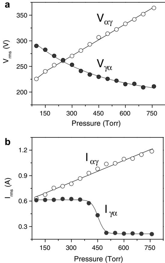
Fig. 4. (a) The transition voltage and (b) current at different gas pressure. Subscripts  $\alpha\gamma$  and  $\gamma\alpha$  denote the  $\alpha$  to  $\gamma$  and  $\gamma$  to  $\alpha$  mode transition, respectively.
