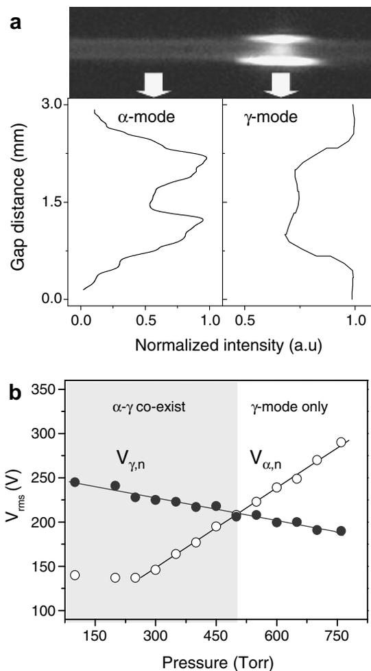
Fig. 2. (a) The normalized visible emission intensity profile of the  $\alpha$ -mode (left) and the  $\gamma$ -mode (right) at 250 Torr when both modes co-exist. (b) Gas pressure effects on the normal glow discharge voltages of the  $\alpha$ -mode ( $-o-$ ,  $V_{\alpha,n}$ ) and the  $\gamma$ -mode ( $-●-$ ,  $V_{\gamma,n}$ ).
