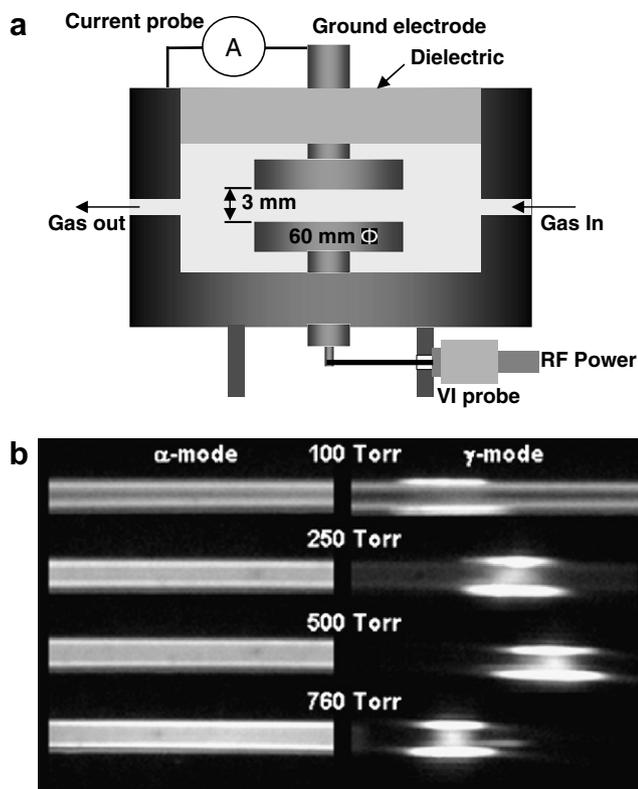
Fig. 1. (a) A Schematic of the experimental setup, and (b) discharge images of the  $\alpha$ - and the  $\gamma$ -modes at 100, 250, 500, and 760 Torr, respectively.
