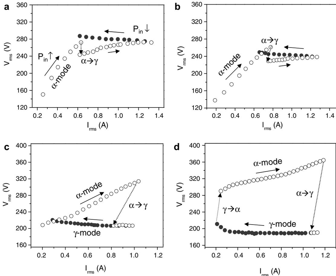
Fig. 3.  $I$ - $V$  curves for (a) 100 Torr, (b) 250 Torr, (c) 500 Torr, and (d) 760 Torr were obtained as increasing (○) and decreasing (●) input power levels denoted as  $P_{in}$ .
