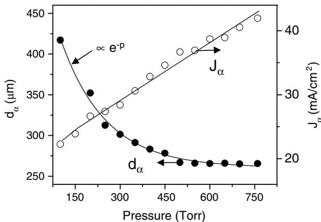
Fig. 5. Dependence of  $\alpha$ -sheath thickness  $d_\alpha$  (—●—) and current density  $J_\alpha$  (—○—) on the gas pressure.  $d_\alpha$  was evaluated from the measured current, voltage, and phase angle using a simple R–C circuit model. As the gas pressure,  $p$ , was raised, linear increase of  $J_\alpha$  ( $J_\alpha \propto p$ ) resulted in an exponential decrease of  $d_\alpha$  ( $d_\alpha \propto e^{-p}$ ).
