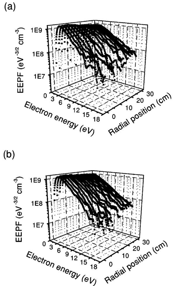
FIG. 9. Radial profiles of the electron probability distribution function obtained simultaneously by two of the probes. The reference sine wave was 1.8  $V_{pp}$  in 7.5 kHz.
