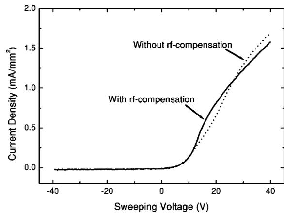
FIG. 6.  $I$ - $V$  characteristic curves obtained from a rf-compensated probe and from a bare probe.
