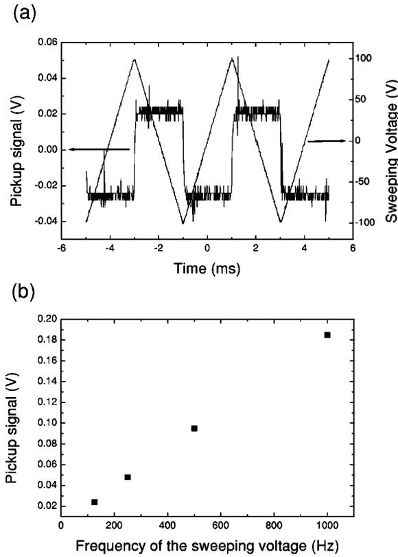
FIG. 4. (a) Differential pickup signal across a 1 k $\Omega$  shunt resistor for 500 Hz, 200  $V_{pp}$  sweeping bias voltage. (b) Amplitude of the pickup signal for 125, 250, 500, and 1000 Hz frequencies of the sweeping voltage.
