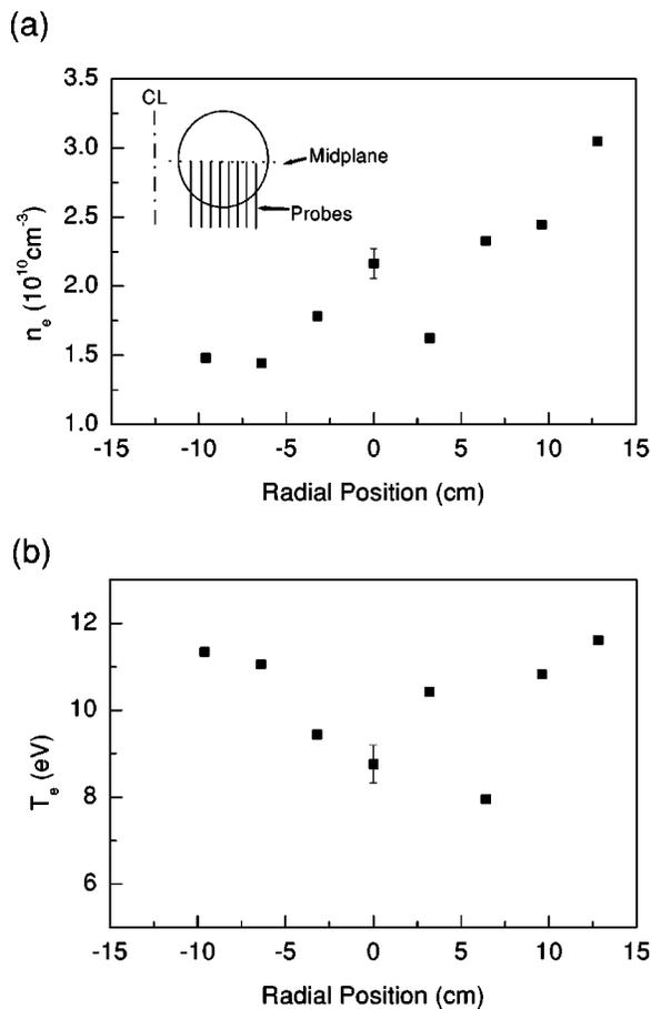
FIG. 10. Radial profile of the (a) electron density and (b) temperature obtained from the  $I$ - $V$  curves simultaneously acquired by the eight Langmuir probes. The plasma was produced by 13.56 MHz, 1 kW rf power input using a toroidally modified Nagoya type III antenna. The zero point of the radial axis corresponds to the geometrical center of the KAIST-TOKAMAK vacuum vessel.
