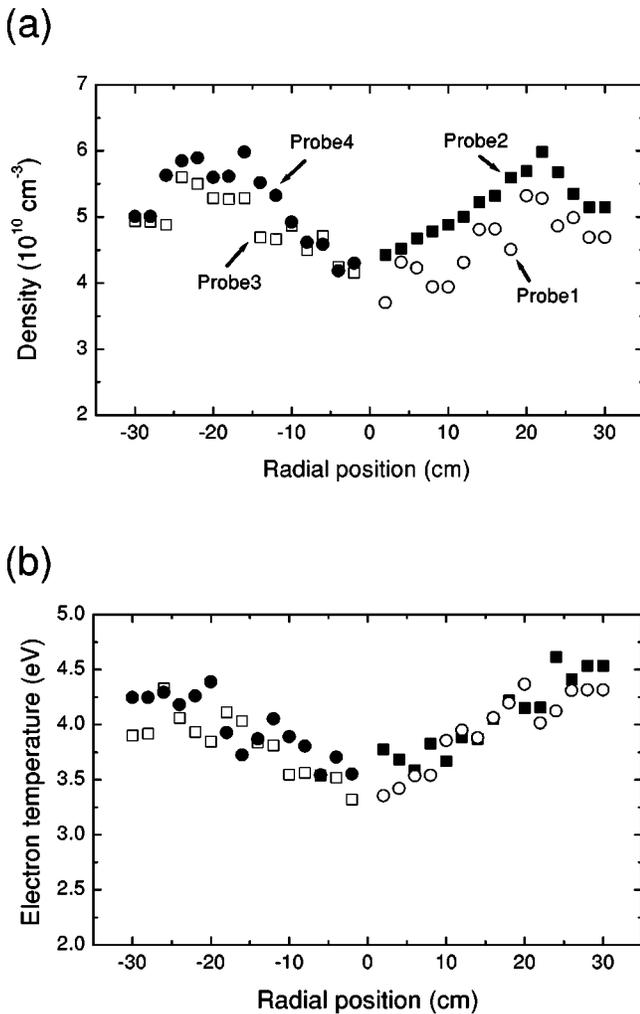
FIG. 8. Radial profiles of the (a) electron density and (b) temperature interpreted from the  $I-V$  curves simultaneously acquired by the four Langmuir probes.
