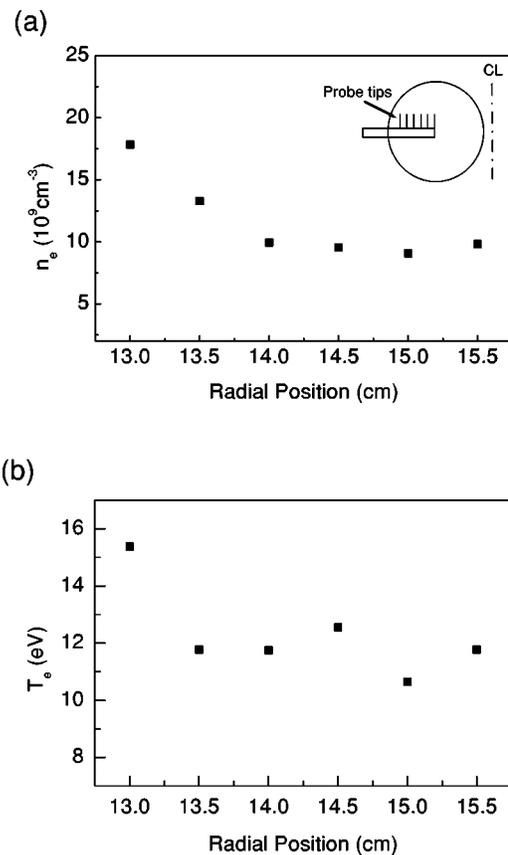
FIG. 11. Radial profile of the (a) electron density and (b) temperature obtained by the six-tip rake probe. The plasma current and toroidal field are 18 kA and 4.5 kG, respectively.
