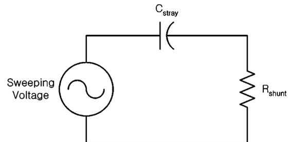
FIG. 3. An equivalent differential circuit consisting of a shunt resistance and the stray capacitance due to the shielding metals and coaxial cables.
