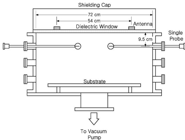
FIG. 5. A schematic drawing of the transformer-coupled plasma source.
