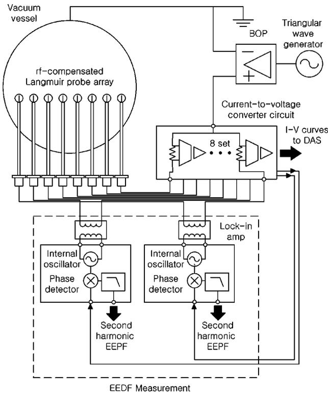
FIG. 1. Schematic diagram of the multichannel Langmuir probe array.
