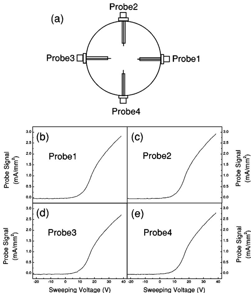
FIG. 7.  $I$ - $V$  curves simultaneously acquired by the four probes installed in the transformer-coupled rf plasma source. The probes were located 22 cm from the radial center, 50  $\Omega$  shunt resistors were used, and the sweeping frequency of the bias voltage was 125 Hz.
