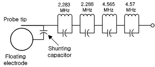
FIG. 2. rf-compensation circuit using a floating electrode and LC resonant filters. The LC resonant filters are tuned to the fundamental and the second harmonic frequency of the rf for plasma generation (2.283 MHz in this case) in order to increase the circuit impedance.
