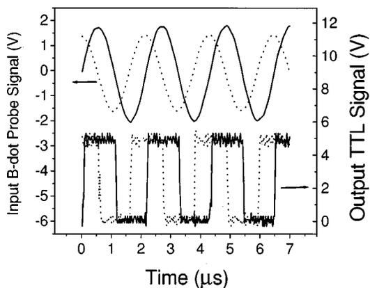
FIG. 3. Sinusoidal IF signals from each B-dot probe (solid and dotted curve) are transformed into TTL signals by the zero-crossing detector. Phase difference between the two IF signals  $\Delta\phi$  is kept unchanged after being transformed into the TTL signals.
