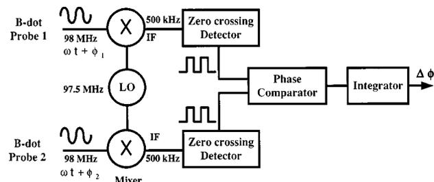
FIG. 1. Schematic diagram of the heterodyne phase detection system. For eliminating electrostatic effects, hybrid combiners are connected between the B-dot probe and the mixer.
