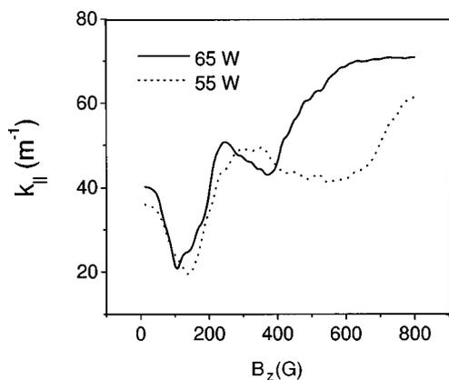
FIG. 6. Real-time measurement of the axial wave number obtained while sweeping the axial magnetic field strength at two different rf powers.
