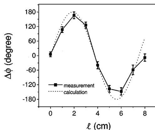
FIG. 5. Phase difference of the helicon wave as a function of the distance between the two B-dot probes. Measurement (solid line) agrees well with the theoretical value (dotted line) calculated from the helicon wave dispersion relation under the experimental condition.
