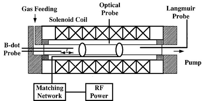
FIG. 4. Schematic diagram of the helicon plasma experimental setup.
