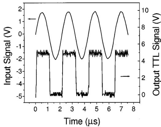
FIG. 2. Input sinusoidal IF signal and the corresponding TTL signal which is the output of the zero-crossing detector.
