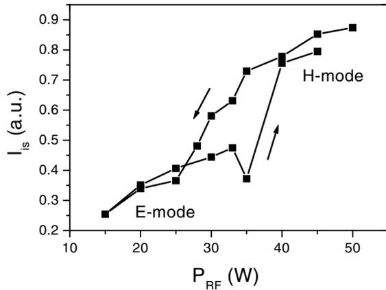
**Figure 3.** E–H transition characteristics shown by Langmuir probe measurement. The ion saturation current versus RF power shows hysteresis near 30 W. The experiment was performed at 1.5 mTorr argon gas pressure and no external magnetic field was applied. A Nagoya type III antenna was used.
