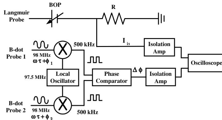
**Figure 2.** Schematic diagram of phase difference and Langmuir probe measurements.
