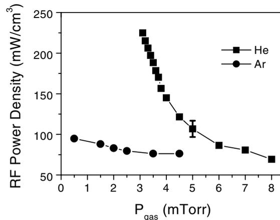
**Figure 8.** RF threshold power density as a function of gas pressure where H–W transition occurs. For helium, the plasma diameter was 1 inch and the applied field was 1.3 kG. A double loop antenna was used. For argon, the plasma diameter was 2 inch with 600 G applied field using a Nagoya type III antenna.
