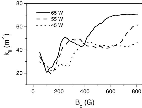
**Figure 9.** Wavenumber measured by a double B-dot probe at different RF power levels. The  $k_{\parallel}$  jump occurs at lower magnetic field as the RF power increases. Argon, 1 mTorr, Nagoya type III antenna.
