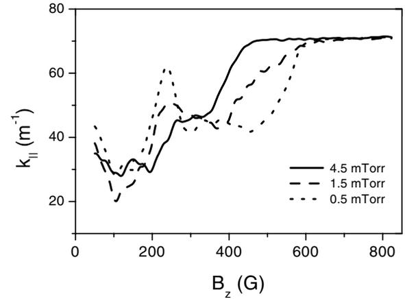
**Figure 10.** Wavenumber measured at different gas pressures. The  $k_{\parallel}$  jump occurs at lower magnetic field as the gas pressure increases at sufficiently high magnetic field ( $B_0 > 500$  G). Argon, 65 W, Nagoya type III antenna.
