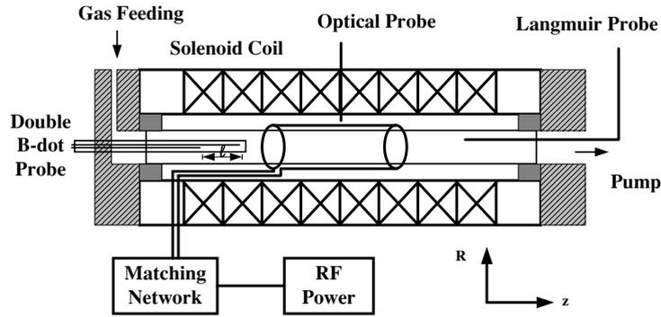
**Figure 1.** Schematic diagram of the helicon plasma source used for experiments. A Nagoya type III antenna is shown.
