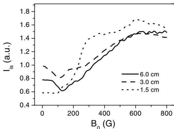
**Figure 7.** Ion saturation current for different antenna lengths. Argon, 65 W, 1.5 mTorr, Nagoya type III antenna.
