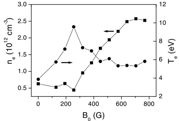
**Figure 4.** The electron density measured by a Langmuir probe shows a density jump near 250 G. The electron temperature increases with field strength at low magnetic field. At 250–300 G, however, it suddenly decreases indicating a dramatic change inside the plasma. Argon, 6 mTorr, 60 W, Nagoya type III antenna.
