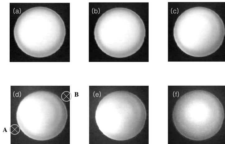
**Figure 5.** Pictures showing the plasma cross section with magnetic field variation. (a) 0 G, (b) 50 G, (c) 80 G, (d) 120 G, (e) <140 G (before transition), (f) >140 G (after transition). A and B denote location of Nagoya type III antenna legs. Argon, 1.5 mTorr, 55 W.
