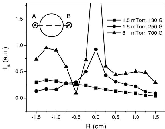
**Figure 6.** Radial profile of the ion saturation current. A and B denote location of Nagoya type III antenna legs. Argon, 65 W, Nagoya type III antenna.
